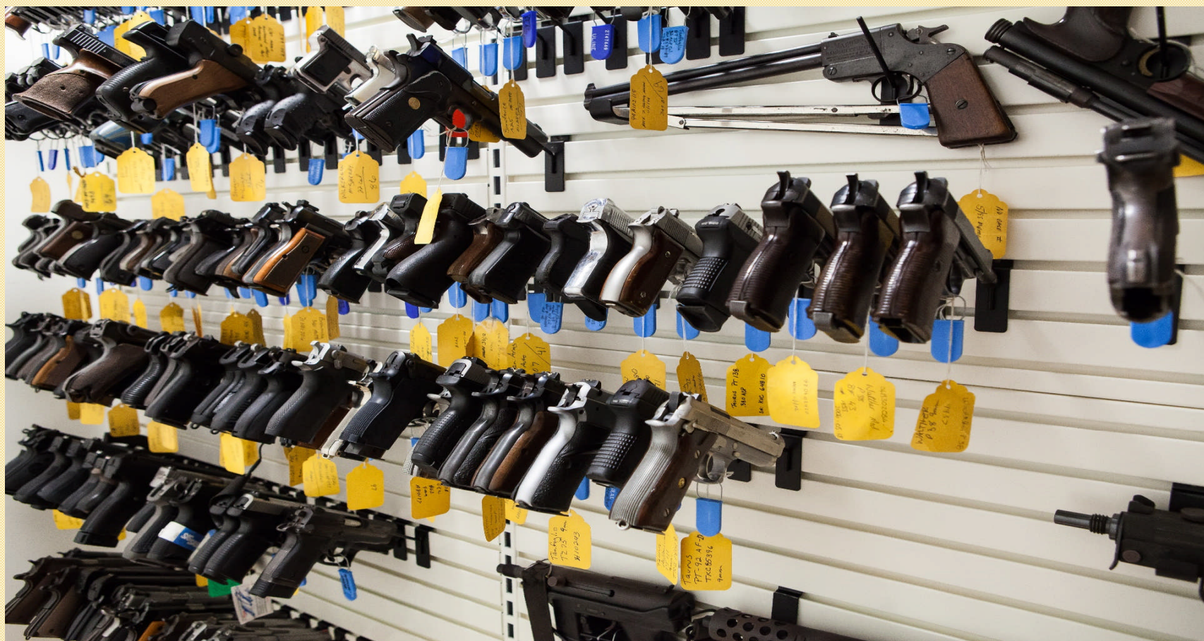
A portion of the firearms that comprise the Laboratory's reference collection; these are used to produce test fires during examination of evidence submitted for Firearms analysis.
