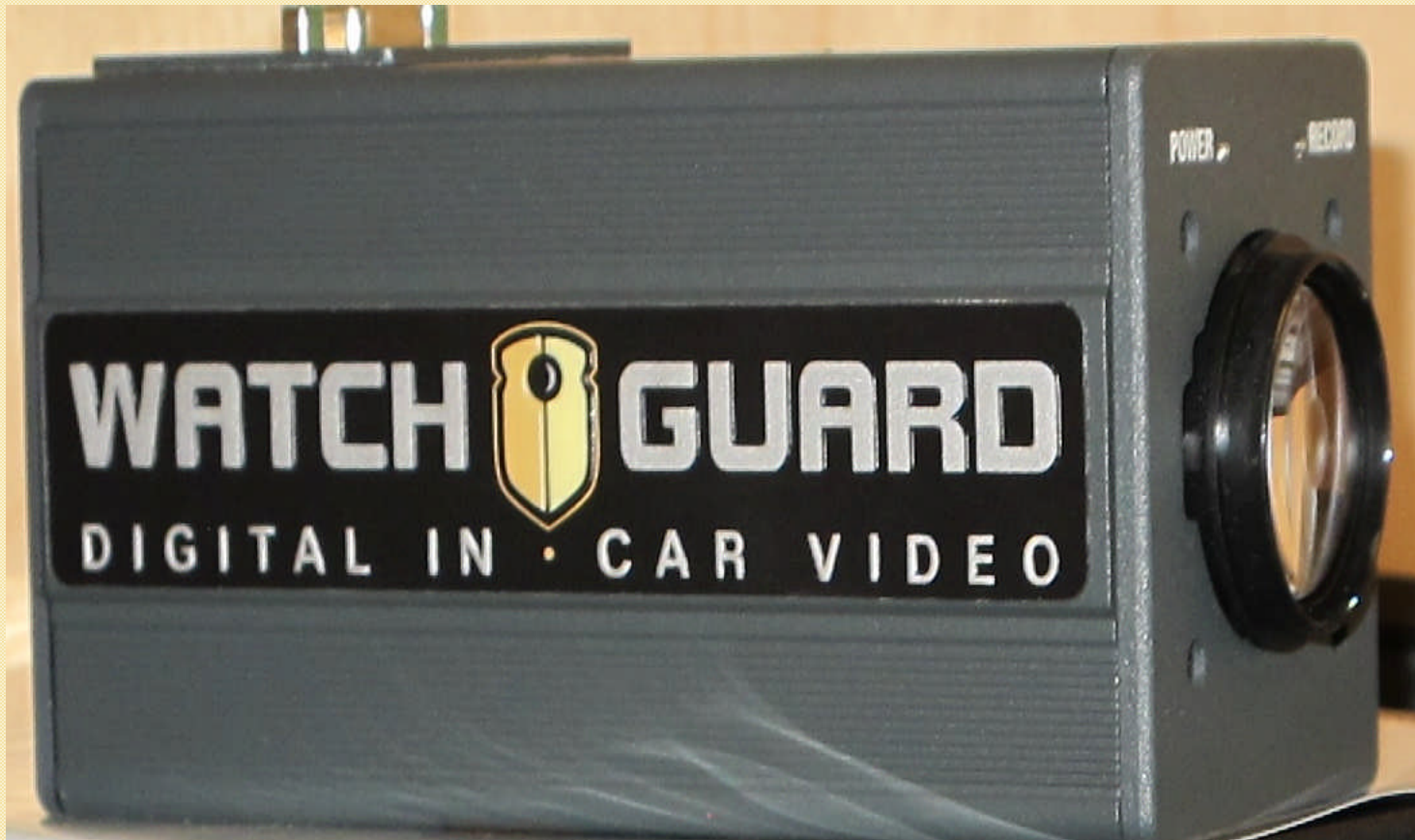
WatchGuard: Current in-car video recording unit utilized by VSP
